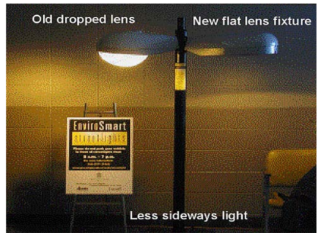
Figure 1.6 Comparison of dropped versus flat lenses
